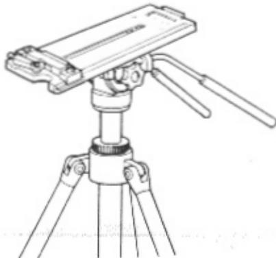
2. While pushing the release button on the lock lever of tripod mounting adaptor, Unlock the lock lever by turning it counterclockwise as shown in the illustration.
