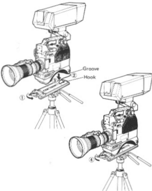
3. Turn the lock lever clockwise as shown illustration until it is locked so that the camera is slid backward to be held on the adaptor firmly.
